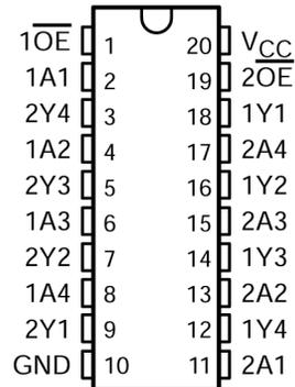
**Figure 4-1. DW or PW Package (Top View)**
