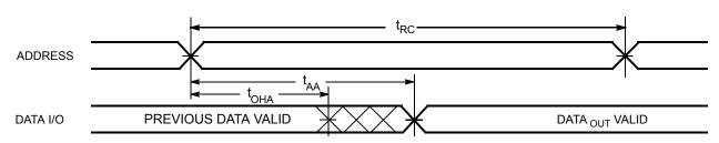
Figure 5. Read Cycle 2 (OE Controlled) [21, 22]
