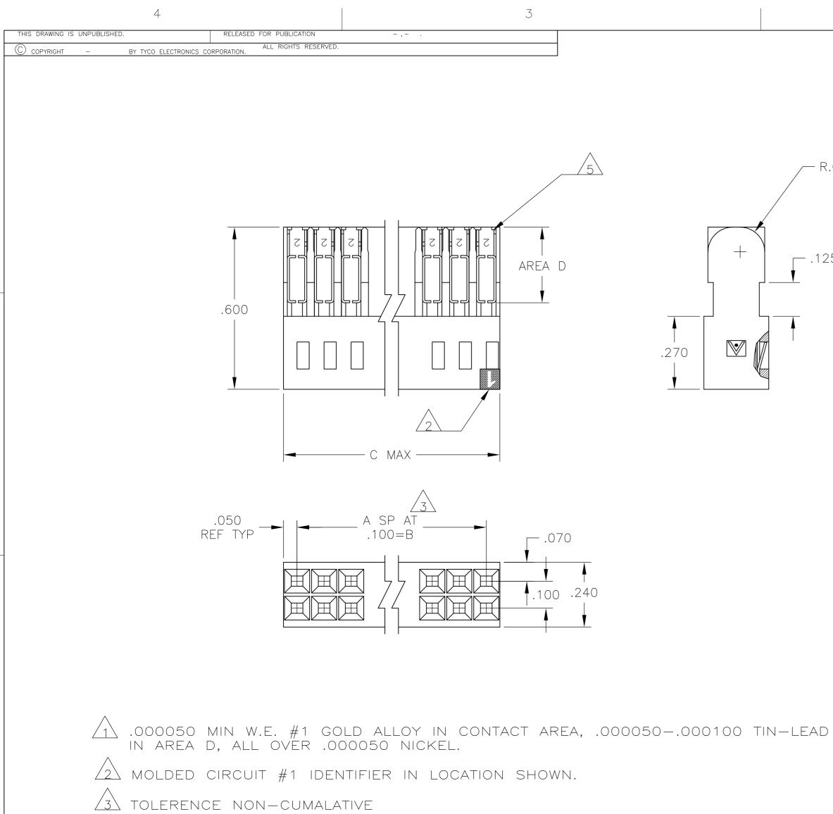
4 USE WITH 22-26 AWG WIRE SIZE, .050 MAX INSULATION DIA., .015 MAX INSULATION WALL THICKNESS.
