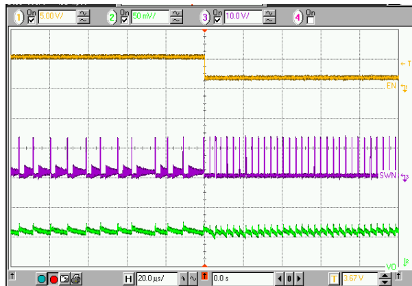
Top to Bottom: EN, SWM, V O Figure 12. On Line Mode Change (DCM → CCM)
