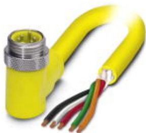
Sensor/actuator cable, 5-position, PVC, yellow, Plug angled 7/8"-16UNF, A-coded, on free cable end, cable length: 2 m
