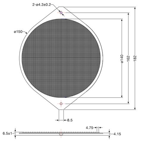
Aluminum/Stainless filters offer high levels of air passage while efficiently filtering contaminants and shielding EMI/RFI.
