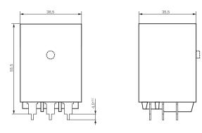
Cover with DIN-snap-on attachement (6.3mm quick connect only) horizontal vertical
