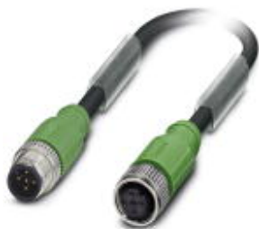
Sensor/actuator cable, 5-position, PUR halogen-free, black-gray RAL 7021, shielded, Plug straight M12, A-coded, on Socket straight M12, A-coded, cable length: 2 m
