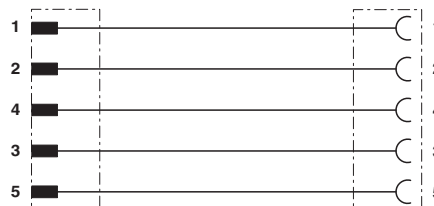
Pin assignment M12 male connector, 5-pos., A-coded, male side
