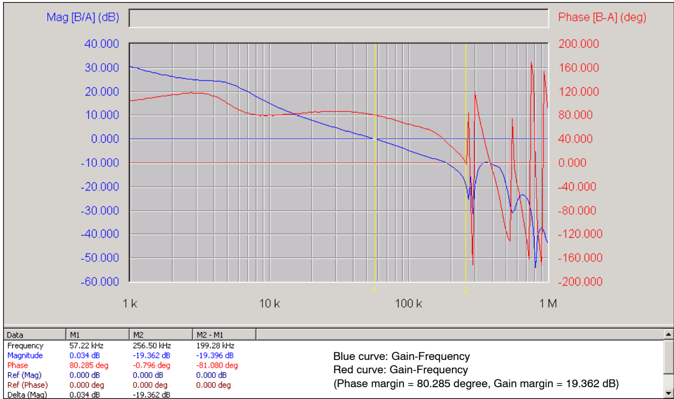
Figure 14. Closed-loop Voltage Loop-gain of the NCP1587E
