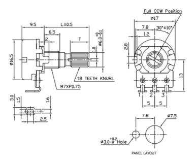
Model P160KN (Side Adjust , PC pins)
