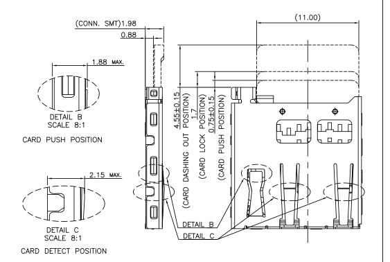
**Card Detection Mechanism:**
