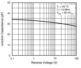
Fig. 5 - Typical Junction Capacitance
