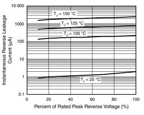
Fig. 4 - Typical Reverse Leakage Characteristics
