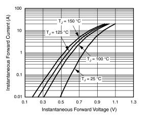
Fig. 3 - Typical Instantaneous Forward Characteristics
