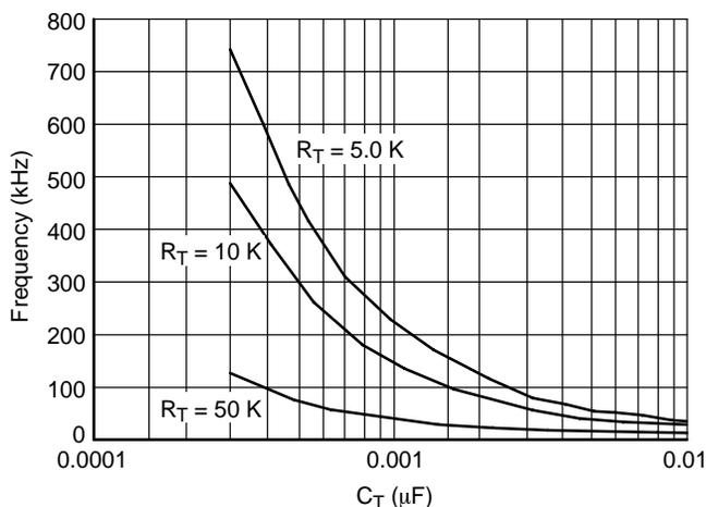
Figure 10. Typical Performance Characteristics, Oscillator Frequency vs.  $C_T$
