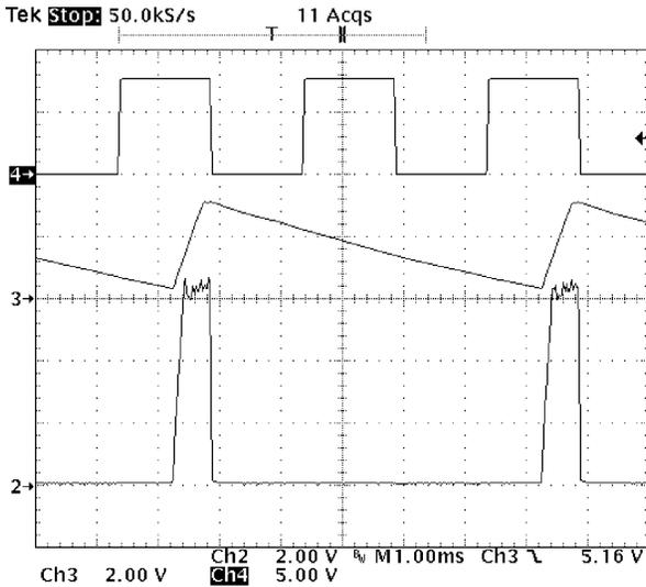
**Figure 6. The Fault Condition Is Triggered when the UV Pin Voltage Falls Below 1.0 V. The Soft–Start Capacitor Is Discharged and the GATE Output Is Disabled. CH2: Envelop of GATE Output, CH3: SS Pin with 0.01  $\mu$ F Capacitor, CH4: UV Pin**
