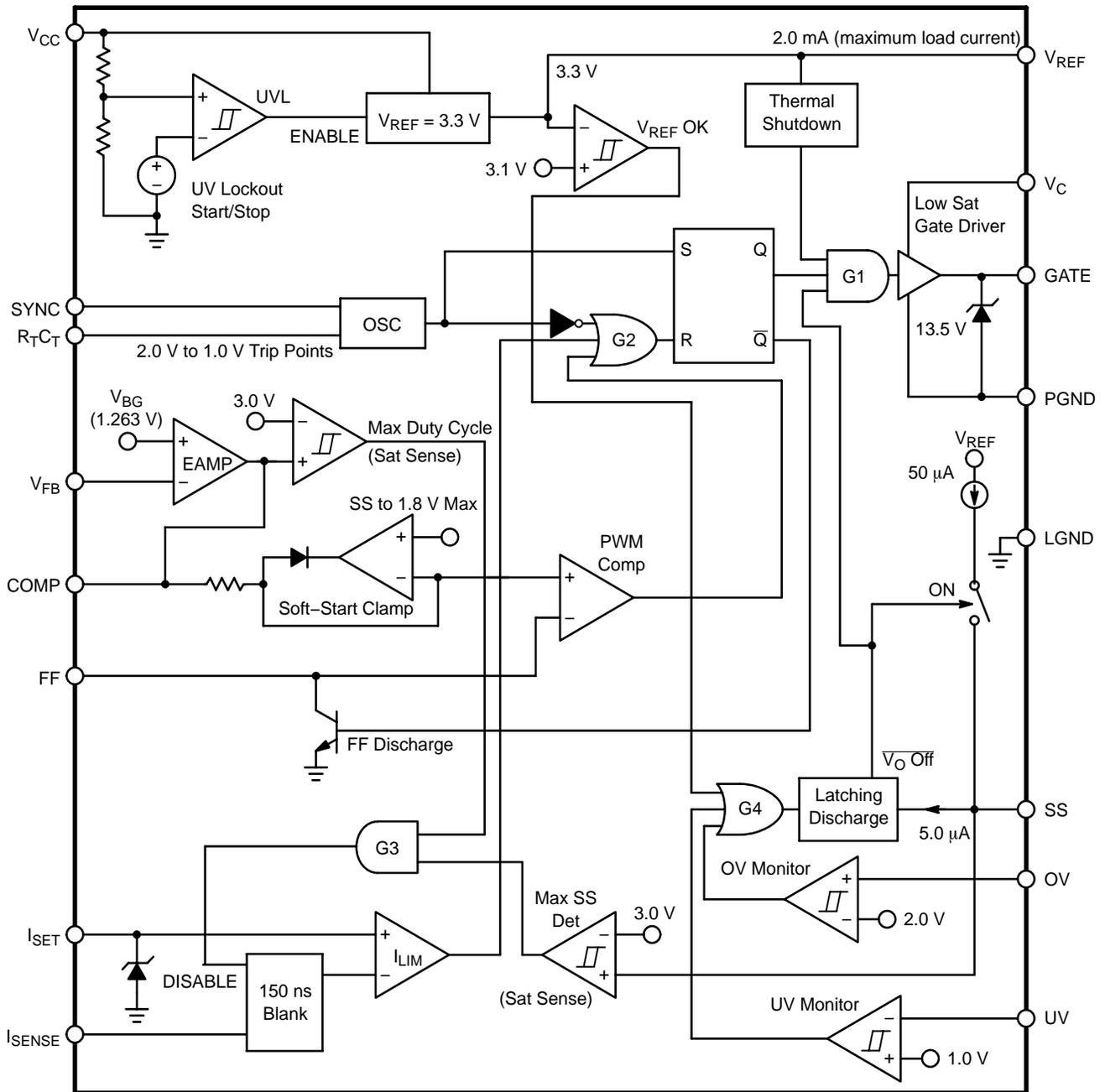
Figure 2. Block Diagram
