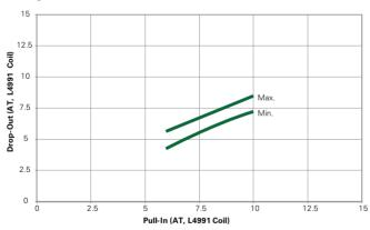
Note: The chart represents the range of Drop-Out, minimum to maximum for a given
