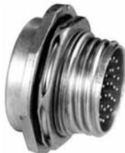
Amphenol® PC Series threaded coupling miniature cylindrical connectors incorporate solder contacts. The PC double stub threaded coupling system cannot be cross threaded, and is mechanically assisted while engaging and disengaging.
