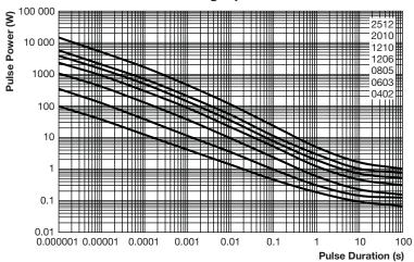
Maximum pulse load, single pulse; applicable if  $\vec{P} \rightarrow 0$  and  $n \le 1000$  and  $\hat{U} \le \hat{U}_{max}$ ; for permissible resistance change equivalent to 8000 h operation
