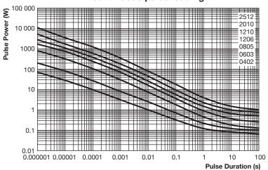
Maximum pulse load, continuous pulses; applicable if  $P \le P(\vartheta_{amb})$  and  $\hat{U} \le \hat{U}_{max}$ ; for permissible resistance change equivalent to 8000 h operation
