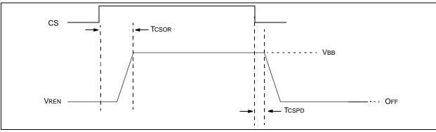
FIGURE 2-6: BUS TO VREN WAKE TIMING DIAGRAM
