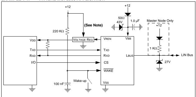
**Note:** For applications with current requirements of less than 20 mA, the connection to +12V can be deleted, and voltage to the regulator supplied directly from the VREN pin.
