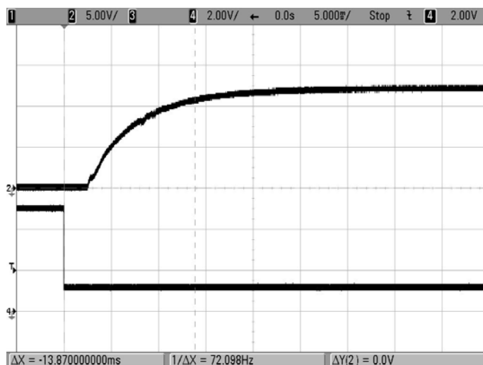
Enable Start-up (Vin=48V, Iout=5A, Cload=1000µF Ta=+25°C) Trace 2=Output, Trace 4= Enable.
