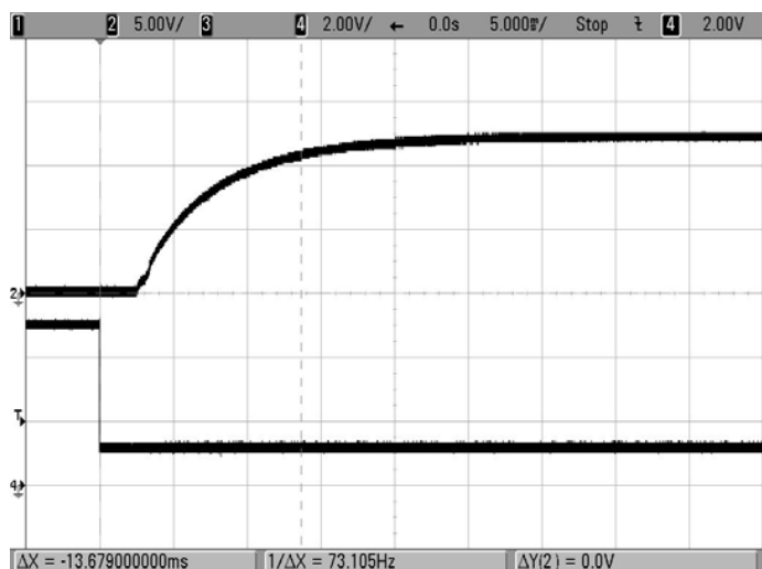
Enable Start-up (Vin=48V, Iout=5A, Cload=1000µF Ta=+25°C) Trace 2=Output, Trace 4= Enable.
