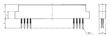
• Recommended board thickness: 0.4 to 0.5mm
