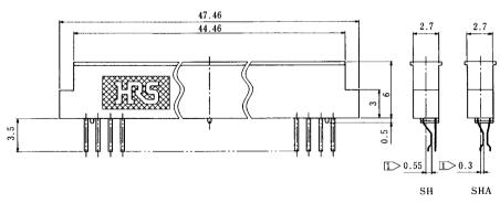
• Recommended board thickness: 0.4 to 0.5mm
