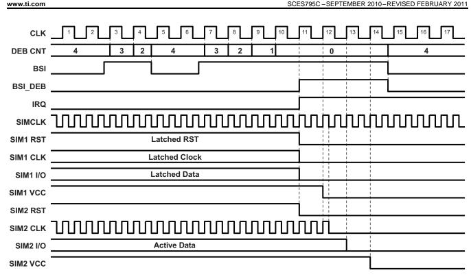
Figure 4. BSI Debounce Timing - SIM1 Isolated, SIM2 Active
