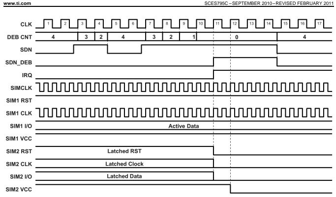
Figure 6. SDN Debounce Timing - SDN Detection Level High
