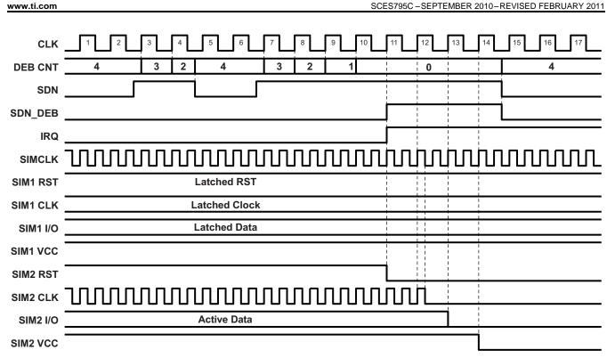
Figure 8. SDN Debounce Timing - SIM1 Isolated and SIM 2 Active
