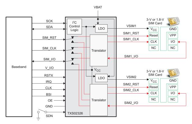
Figure 1. Interfacing With SIM Card
