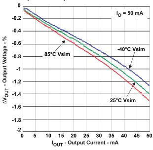
Figure 13. Load Regulation, lout = 50 mA, Class-C
