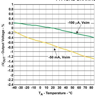
Figure 12. Output Voltage vs Temperature, Class-B/C
