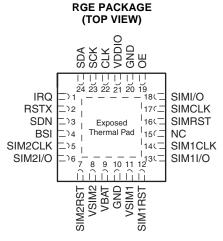
Note: The Exposed Thermal Pad must be connect to Ground.
