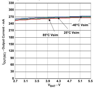
Figure 16. Line Regulation, lout = 50 mA, Class-B
