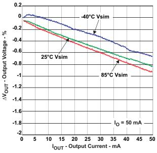
Figure 14. Load Regulation, lout = 50 mA, Class-B
