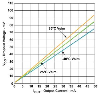
Figure 11. Dropout Voltage vs Output Current
