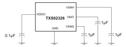
Figure 9. Typical Application circuit for TXS02326
