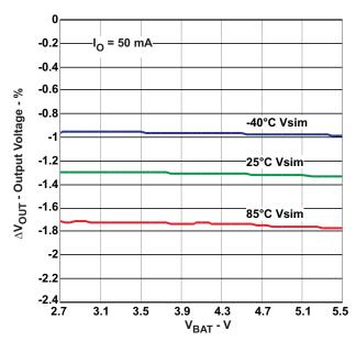
Figure 15. Line Regulation, lout = 50 mA, Class-C
