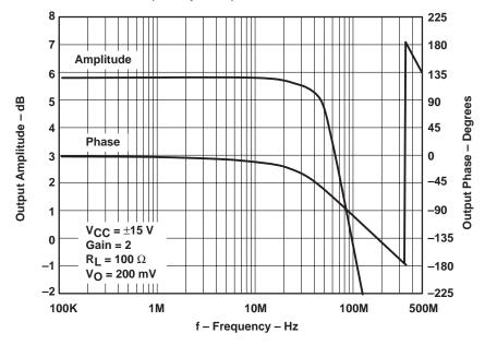
Figure 1–4 shows the typical frequency response of the THS4061 EVM using the inverting input (G = –1). Typical –0.1 dB bandwidths are 12 MHz and a –3-dB bandwidth of 65 MHz with a  $\pm$  15 V power supply. These bandwidths remain consistent when the power supply drops to  $\pm$ 5 V.
