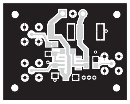
Figure 2–2. THS4061 EVM PC Board Layout – Component Side
