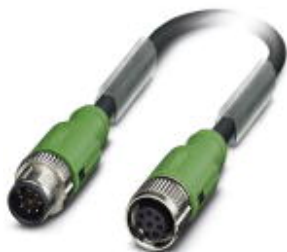
Sensor/actuator cable, 8-position, PUR halogen-free, black-gray RAL 7021, shielded, Plug straight M12 SPEEDCON, on Plug straight M12 SPEEDCON, cable length: 3.5 m
