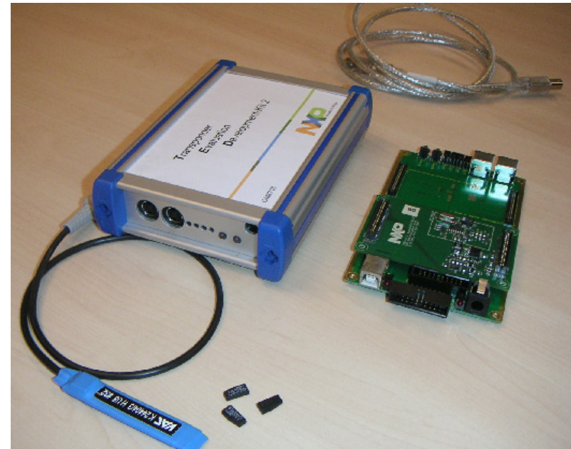
OM6716 - TED-Kit2 comes in metal casing (easy upgrade of containing boards due to stacked Xboard concept)
