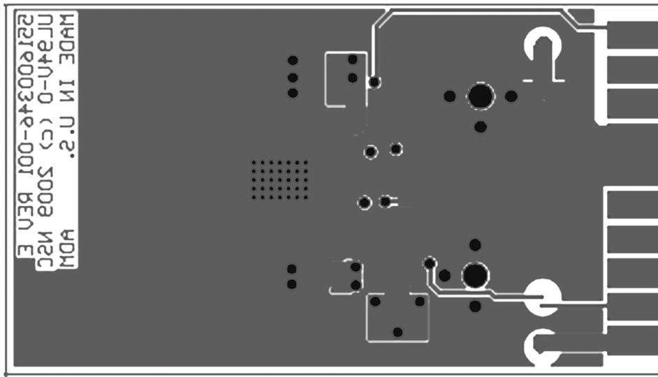
Figure 5. Bottom Layer (Ground and Routing)
