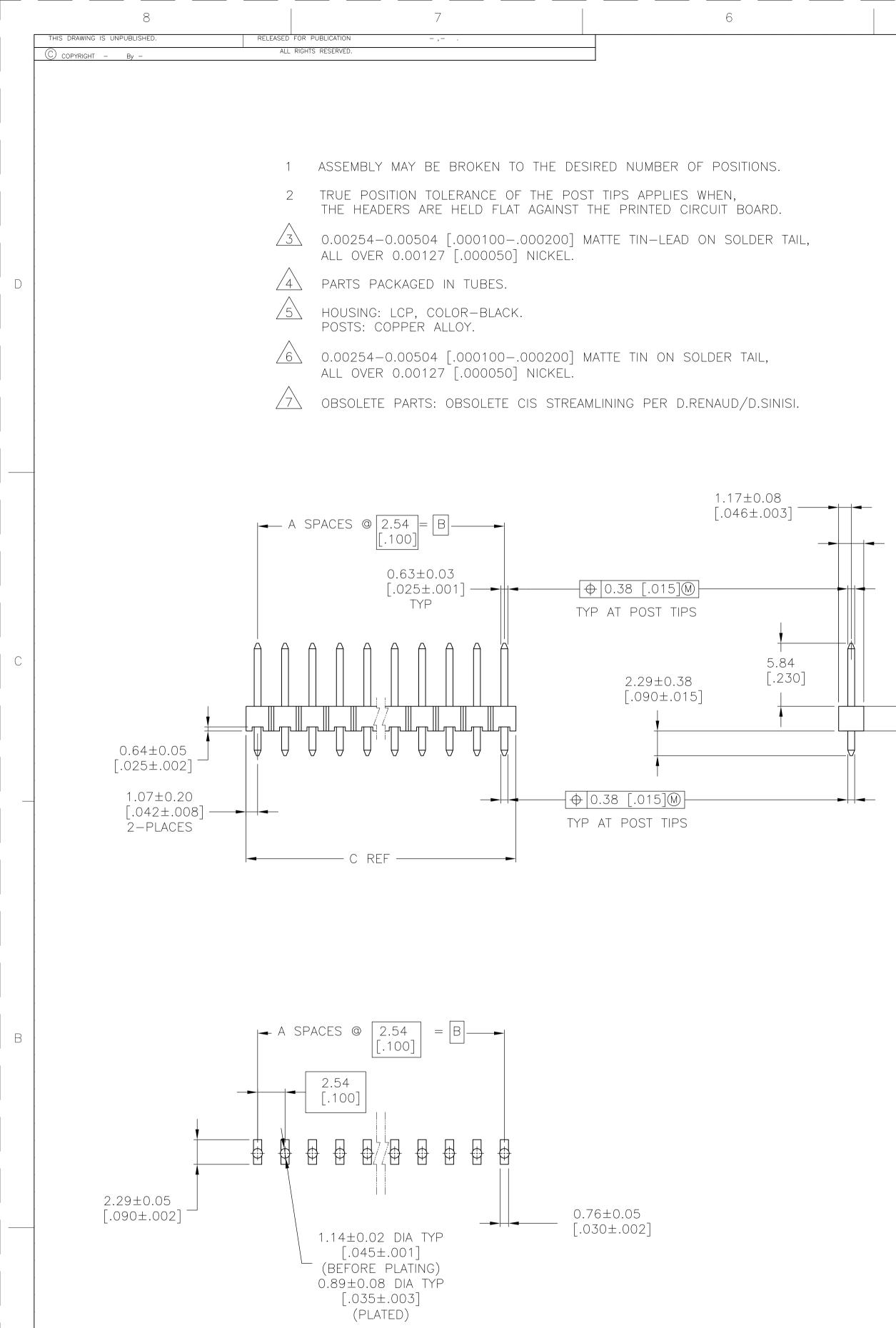
RECOMMENDED PC BOARD MOUNTING DIMENSIONS FOR .063 [1.60] THICK PC BOARD AND .012 [.305] STENCIL THICK.
