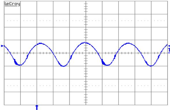
Figure 13. Input reflected ripple-current,  $i_c$  (200 mA/div.), measured at input terminals at full rated load current and  $V_{in} = 48$  V. Refer to Figure 11 for test setup. Time scale: 1  $\mu$ s/div.
