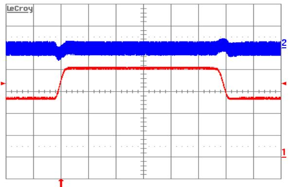
Figure 8. Output voltage response to load current step-change (12.5A–18.75A–12.5A) at  $V_{in} = 48\text{ V}$ . Top trace: output voltage (100mV/div.). Bottom trace: load current (5A/div.). Current slew rate: 0.1A/µs.  $C_o = 1\mu\text{F cer} + 10\mu\text{F tant}$ . Time scale: 0.2ms/div.
