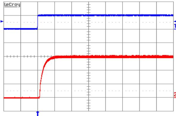
Figure 6. Turn-on transient at full rated load current (resistive) with no output capacitor at  $V_{in} = 48\text{ V}$ , triggered via ON/OFF pin. Top trace: ON/OFF signal (5 V/div.). Bottom trace: Output voltage (0.5 V/div.). Time scale: 5 ms/div.
