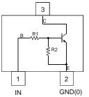
Schematic and Pin Configuration
