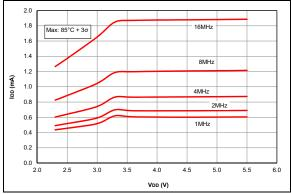
FIGURE 37-22: IDD Maximum, HFINTOSC Mode, PIC16F1764/5/8/9 Only.
