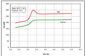
**FIGURE 37-18:** IDD, MFINTOSC Mode, Fosc = 500 kHz, PIC16F1764/5/8/9 Only.
