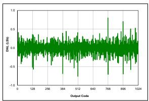
FIGURE 37-77: ADC 10-Bit Mode, Single-Ended DNL, VDD = 3.0V,  $TAD = 1 \mu S$ ,  $25^{\circ}C$ .
