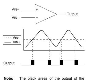
The black areas of the output of the comparator represent the uncertainty due to input offsets and response time.
