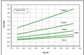
FIGURE 37-19: IDD Typical, HFINTOSC Mode, PIC16LF1764/5/8/9 Only.
