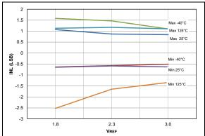
**FIGURE 37-84:** ADC 10-Bit Mode, Single-Ended INL, VDD = 3.0V, TAD = 1  $\mu$ S.
