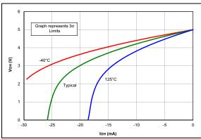
FIGURE 37-45: Standard IO VOH vs. IOH Over Temperature, VDD = 5.0V, PIC16F1764/5/8/9 Only.
