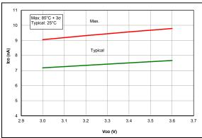
**FIGURE 37-33:** IPD, Brown-Out Reset (BOR), BORV = 1, PIC16LF1764/5/8/9 Only.
