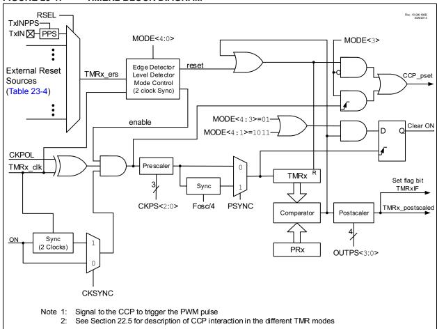
FIGURE 23-2: TIMER2 CLOCK SOURCE BLOCK DIAGRAM
