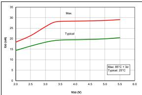
FIGURE 37-32: IPD, Fixed Voltage Reference (FVR), PIC16F1764/5/8/9 Only.
