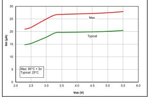
**FIGURE 37-16:** IDD LFINTOSC Mode, Fosc = 31 kHz, PIC16F1764/5/8/9 Only.
