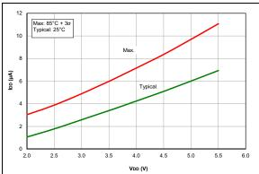
FIGURE 37-38: IPD, Timer1 Oscillator, Fosc = 32 kHz, PIC16F1764/5/8/9 Only.
