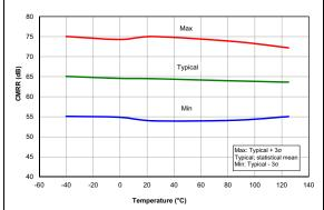
**FIGURE 37-94:** Op Amp, Common Mode Rejection Ratio (CMRR), VDD = 3.0V.
