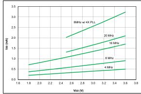
**FIGURE 37-23:** IDD Typical, HS Oscillator, 25°C, PIC16LF1764/5/8/9 Only.
