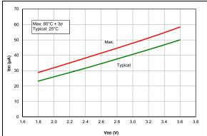
FIGURE 37-7: IDD, EC Oscillator LP Mode, Fosc = 500 kHz, PIC16LF1764/5/8/9 Only.
