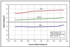
FIGURE 37-96: Op Amp, Offset Over Common Mode Voltage, VDD = 3.0V, Temp. = 25°C.
