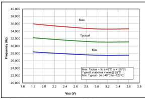
FIGURE 37-57: LFINTOSC Frequency, PIC16LF1764/5/8/9 Only.
