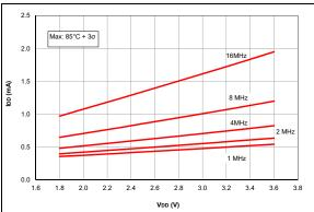
FIGURE 37-20: IDD Maximum, HFINTOSC Mode, PIC16LF1764/5/8/9 Only.
