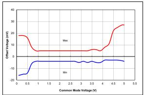
FIGURE 37-109: Comparator Offset, NP Mode (CxSP = 1), VDD = 5.5V, Typical Measured Values from -40°C to 125°C, PIC16F1764/5/8/9 Only.
