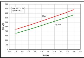
FIGURE 37-9: IDD Typical, EC Oscillator MP Mode, Fosc = 4 MHz, PIC16LF1764/5/8/9 Only.
