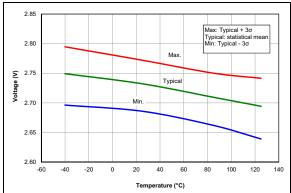
**FIGURE 37-65:** Brown-Out Reset Voltage, High Trip Point (BORV = 0).
