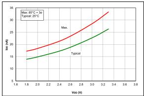
FIGURE 37-31: IPD, Fixed Voltage Reference (FVR), PIC16LF1764/5/8/9 Only.
