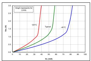
**FIGURE 37-54:** Vol vs. Iol Over Temperature, VDD = 3.0V.
