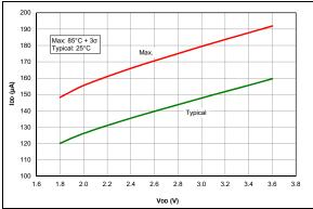
FIGURE 37-17: IDD, MFINTOSC Mode, Fosc = 500 kHz, PIC16LF1764/5/8/9 Only.
