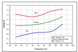
FIGURE 37-73: POR Rearm Voltage, NP Mode, PIC16LF1764/5/8/9 Only.
