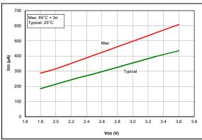
FIGURE 37-3: IDD, XT Oscillator 4 MHz, PIC16LF1764/5/8/9 Only.
