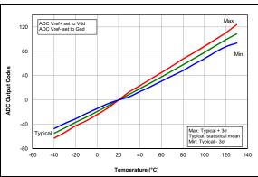
FIGURE 37-92: Temp. Indicator Slope Normalized to 20°C, Low Range, VDD = 3.0V, PIC16LF1764/5/8/9 Only.
