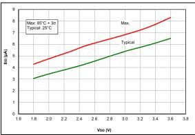
FIGURE 37-15: IDD LFINTOSC Mode, Fosc = 31 kHz, PIC16LF1764/5/8/9 Only.
