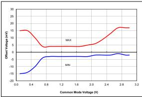
**FIGURE 37-105:** Comparator Offset, NP Mode (CxSP = 1), VDD = 3.0V, Typical Measured Values at 25°C.
