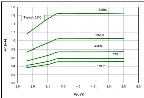
FIGURE 37-21: IDD Typical, HFINTOSC Mode, PIC16F1764/5/8/9 Only.
