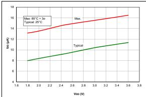
FIGURE 37-1: IDD, LP Oscillator Mode, Fosc = 32 kHz, PIC16LF1764/5/8/9 Only.
