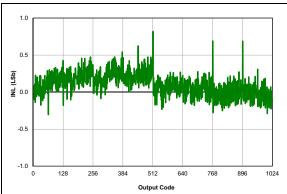
**FIGURE 37-80:** ADC 10-Bit Mode, Single-Ended INL, VDD = 3.0V,  $TAD = 4 \mu S$ ,  $25^{\circ}C$ .
