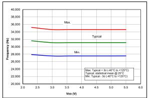
FIGURE 37-58: LFINTOSC Frequency, PIC16F1764/5/8/9 Only.
