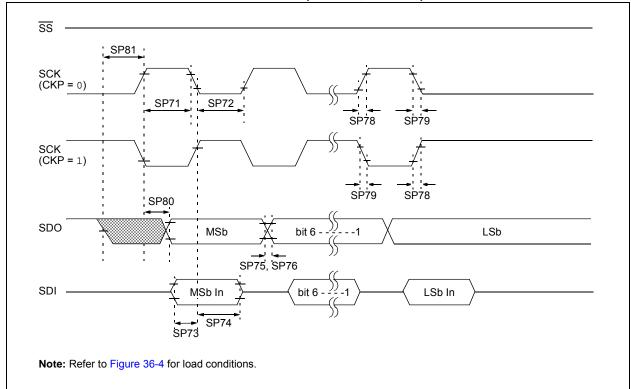
FIGURE 36-18: SPI MASTER MODE TIMING (CKE = 1, SMP = 1)
