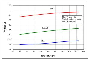
FIGURE 37-67: LPBOR Reset Voltage.
