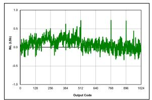
FIGURE 37-79: ADC 10-Bit Mode, Single-Ended INL, VDD = 3.0V,  $TAD = 1 \mu S$ ,  $25^{\circ}C$ .
