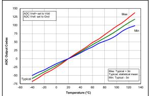
FIGURE 37-88: Temp. Indicator Slope Normalized to 20°C, High Range, VDD = 5.5V, PIC16F1764/5/8/9 Only.
