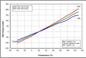
FIGURE 37-89: Temp. Indicator Slope
