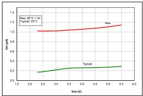
**FIGURE 37-42:** IPD, ADC Non-Converting, PIC16F1764/5/8/9 Only.
