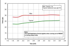
FIGURE 37-76: FVR Stabilization Period, PIC16LF1764/5/8/9 Only.
