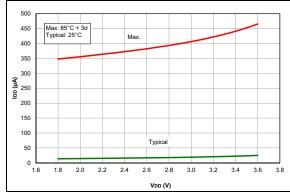
FIGURE 37-41: IPD, ADC Non-Converting, PIC16LF1764/5/8/9 Only.
