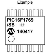
20-Lead SOIC (7.50 mm)
