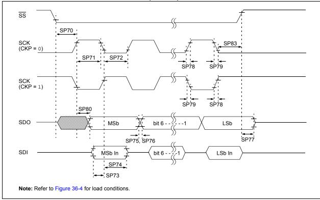
FIGURE 36-20: SPI SLAVE MODE TIMING (CKE = 1)
