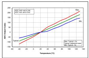
FIGURE 37-91: Temp. Indicator Slope Normalized to 20°C, Low Range, VDD = 1.8V, PIC16LF1764/5/8/9 Only.
