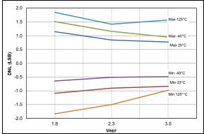
**FIGURE 37-83:** ADC 10-Bit Mode, Single-Ended DNL, VDD = 3.0V, TAD = 1  $\mu$ S.
