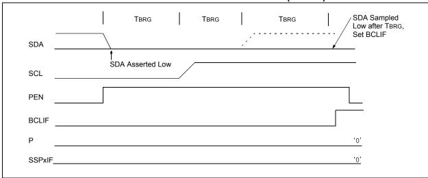
FIGURE 32-39: BUS COLLISION DURING A STOP CONDITION (CASE 2)
