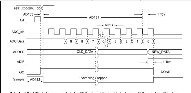
Note 1: If the ADC clock source is selected as FRC, a time of TcY is added before the ADC clock starts. This allows the SLEEP instruction to be executed.
