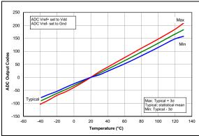
FIGURE 37-93: Temp. Indicator Slope Normalized to 20°C, High Range, VDD = 3.6V, PIC16LF1764/5/8/9 Only.
