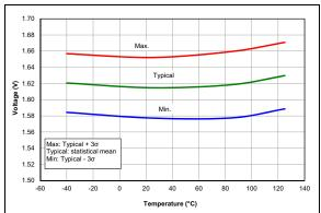
FIGURE 37-71: POR Release Voltage.
