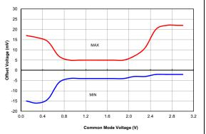
**FIGURE 37-106:** Comparator Offset, NP Mode (CxSP = 1), VDD = 3.0V, Typical Measured Values From -40°C to 125°C.
