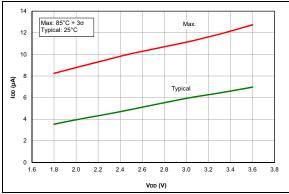
FIGURE 37-5: IDD, EC Oscillator LP Mode, Fosc = 32 kHz, PIC16LF1764/5/8/9 Only.
