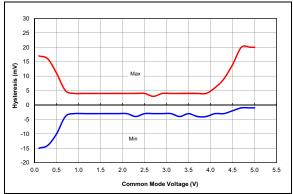
FIGURE 37-108: Comparator Offset, NP Mode (CxSP = 1), VDD = 5.0V, Typical Measured Values at 25°C, PIC16F1764/5/8/9 Only.
