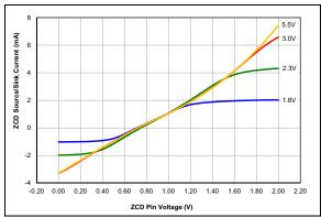
**FIGURE 37-120:** ZCD Pin Current Over ZCD Pin Voltage, Typical Measured Values from -40°C to 125°C.
