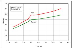
FIGURE 37-10: IDD Typical, EC Oscillator MP Mode, Fosc = 4 MHz, PIC16F1764/5/8/9 Only.
