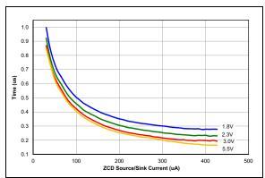
FIGURE 37-121: ZCD Pin Response Time Over Current, Typical Measured Values from -40°C to 125°C.
