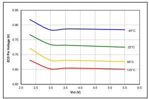
FIGURE 37-118: ZCD Pin voltage, Typical Measured Values.
