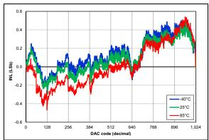
FIGURE 37-115: Typical INL Error, VDD = 3.6V, VREF = VDD.
