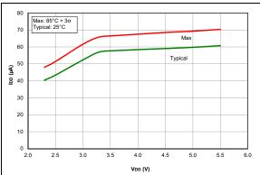
FIGURE 37-8: IDD, EC Oscillator LP Mode, Fosc = 500 kHz, PIC16F1764/5/8/9 Only.
