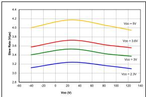
FIGURE 37-101: Op Amp, Output Slew Rate, Falling Edge.
