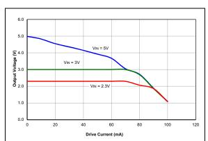
**FIGURE 37-102:** Op Amp, Output Drive Strength, VDD = 5.0V, Temp. = 25°C, PIC16F1764/5/8/9 Only.
