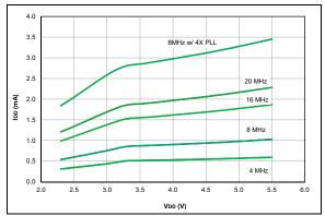
**FIGURE 37-25:** IDD Typical, HS Oscillator, 25°C, PIC16F1764/5/8/9 Only.
