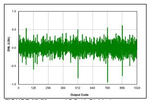
**FIGURE 37-78:** ADC 10-Bit Mode, Single-Ended DNL, VDD = 3.0V,  $TAD = 4 \mu S$ ,  $25^{\circ}C$ .
