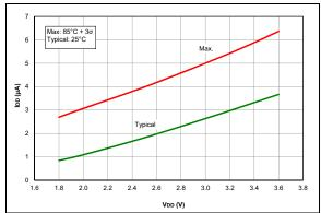
**FIGURE 37-37:** IPD, Timer1 Oscillator, Fosc = 32 kHz, PIC16LF1764/5/8/9 Only.
