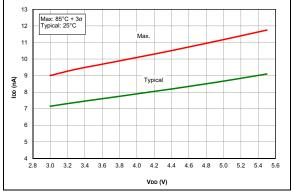
**FIGURE 37-34:** IPD, Brown-Out Reset (BOR), BORV = 1, PIC16F1764/5/8/9 Only.
