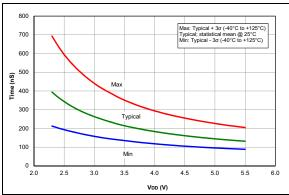
FIGURE 37-113: Comparator Output Filter
