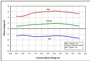
FIGURE 37-97: Op Amp, Offset Over Common Mode Voltage, VDD = 5.0V, Temp. = 25°C, PIC16F1764/5/8/9 Only.
