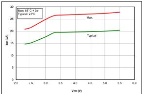
**FIGURE 37-6:** IDD, EC Oscillator LP Mode, Fosc = 32 kHz, PIC16F1764/5/8/9 Only.
