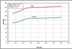
**FIGURE 37-2:** IDD, LP Oscillator Mode, Fosc = 32 kHz, PIC16F1764/5/8/9 Only.
