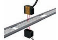
Checking for doubled-up lead frames
