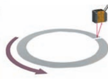
Checking welding point positions on ring gears
