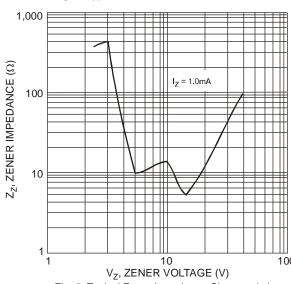
Fig. 5 Typical Zener Impedance Characteristics
