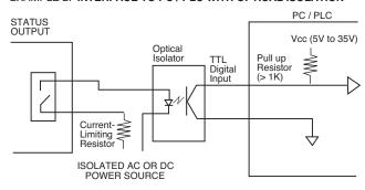
Note: When energized (switch in the "on" position), a low load terminal voltage will be present when fuses are open or when pullout module is removed. The leakage current is limited to .5mA maximum.
