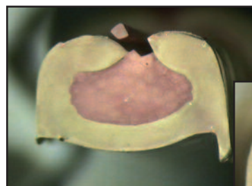
Visible Deformation of Outer Crimp Surface as a result of Indentation from Material Buildup on Crimper
