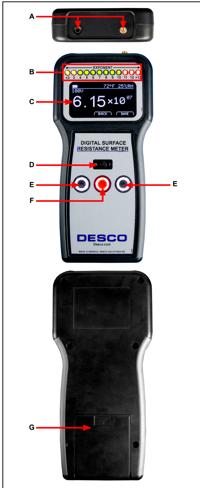
Figure 4. Digital Surface Resistance Meter features and components
