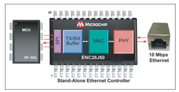
Microchip addresses the growing demand for a small and low-cost embedded Ethernet solution by offering the following:
