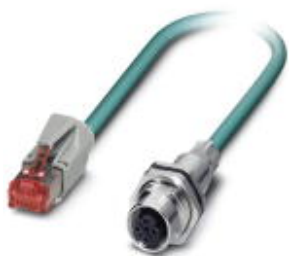
Assembled Ethernet cable, CAT5e, shielded, 2-pair, 26 AWG stranded (7-wire), RAL 5021 (water blue), M12 flush-type socket, rear/screw mounting with SPEEDCON to RJ45 plug/IP20, line, length 5 m
