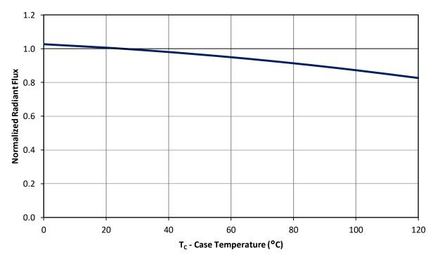
Figure 8: Typical normalized radiant flux vs. case temperature.
