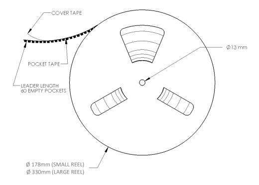
Figure 13: Emitter reel specifications (mm).
