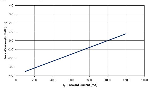
Figure 9: Typical peak wavelength shift vs. forward current @  $T_{\text{C}}$  = 25°C.
