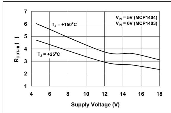
**FIGURE 2-11:** Output Resistance (Output High) vs. Supply Voltage.
