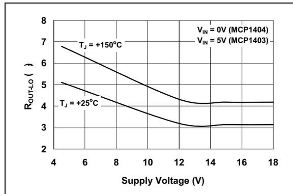
**FIGURE 2-12:** Output Resistance (Output Low) vs. Temperature.
