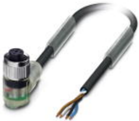
Sensor/actuator cable, 4-position, PUR, black-gray RAL 7021, free cable end, on Socket angled M12, A-coded, with 3 LEDs, cable length: 10 m
