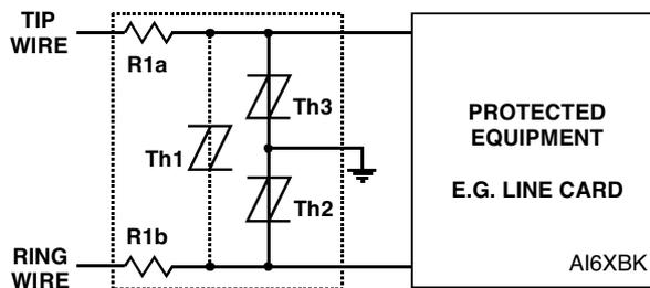
Figure 15. Protection Module
