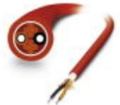
Highly flexible POF round cable for use in drag chains for an alternating bending frequency of up to 5 million cycles with individual elements made of highly wear-resistant polyamide (PE). The cable is halogen-free, ozone and UV resistant and has a rugged polyurethane (PUR) outer sheath.
