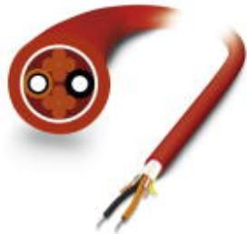
Polymer fiber cable, duplex 980/1000 µm, heavy-weight, highly flexible version for flexible conduit applications, by the meter, without connector
