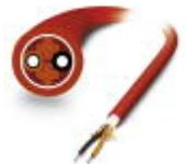
Highly flexible POF round cable (IP20 heads only) for use in drag chains. Individual elements made from extremely wear-resistant polyamide (PE). The cable is halogen-free, ozone and UV resistant, and has a rugged polyurethane (PUR) outer sheath.
