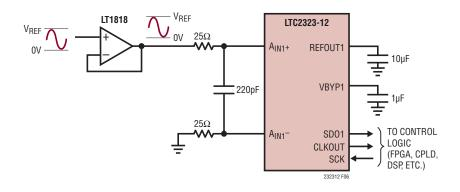
Figure 6. Pseudo-Differential Unipolar Application Circuit
