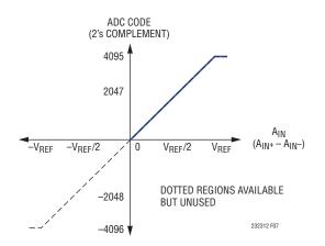
Figure 7. Pseudo-Differential Unipolar Transfer Function
