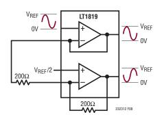
Figure 8. Single-Ended to Differential Driver
