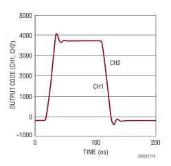
Figure 15. Transient Response of the LTC2323-12
