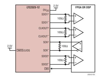
Figure 22. LTC2323 Using the LVDS Interface
