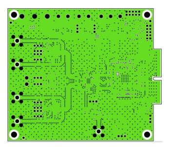
Figure 24. Layer 2, Ground Plane
