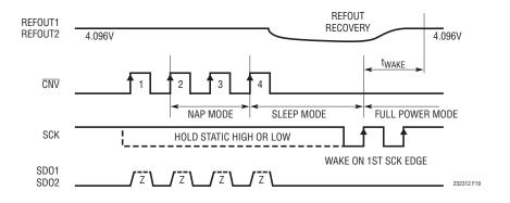
Figure 19. CMOS Mode SLEEP and WAKE Using SCK
