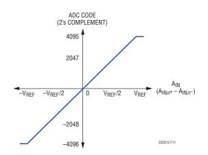
Figure 11. Fully-Differential Transfer Function
