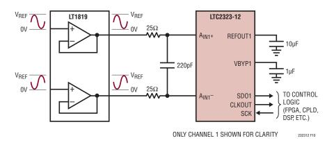
Figure 10. Fully-Differential Application Circuit
