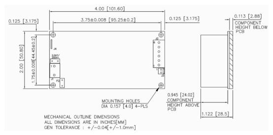
Figure 2. Mechanical Drawing MBC40-1xxxG
