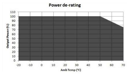
Figure 1. Derating Curve
