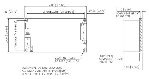
Figure 3. Mechanical Drawing MBC40-3xxxG
