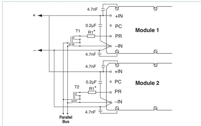
Figure 10 — Transformer-coupled interface
