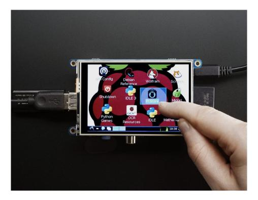
Is this not the cutest, little display for the Raspberry Pi? It features a **3.5"** display with **480x320** 16-bit color pixels and a resistive touch overlay, but is only slightly larger than our popular original (https://adafru.it/dDE). The plate uses the high speed SPI interface on the Pi and can use the mini display as a console, X window port, displaying images or video etc. Best of all it plugs right in on top!
