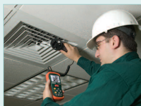
AN100 and AN200 used in HVAC applications measuring airflow from heating vents.
