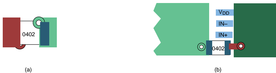
Figure 27. Typical Decoupling Capacitor Layouts
