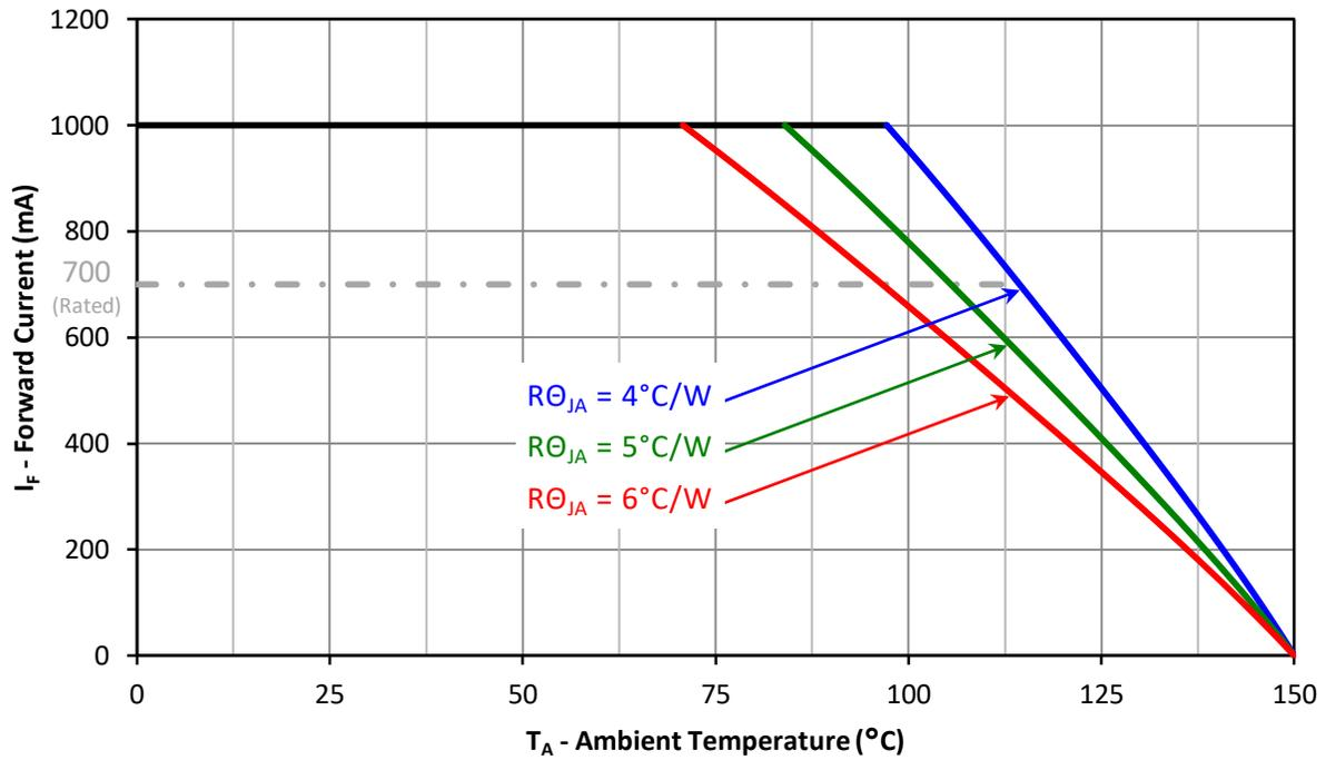
Figure 11: Maximum forward current vs. ambient temperature.
