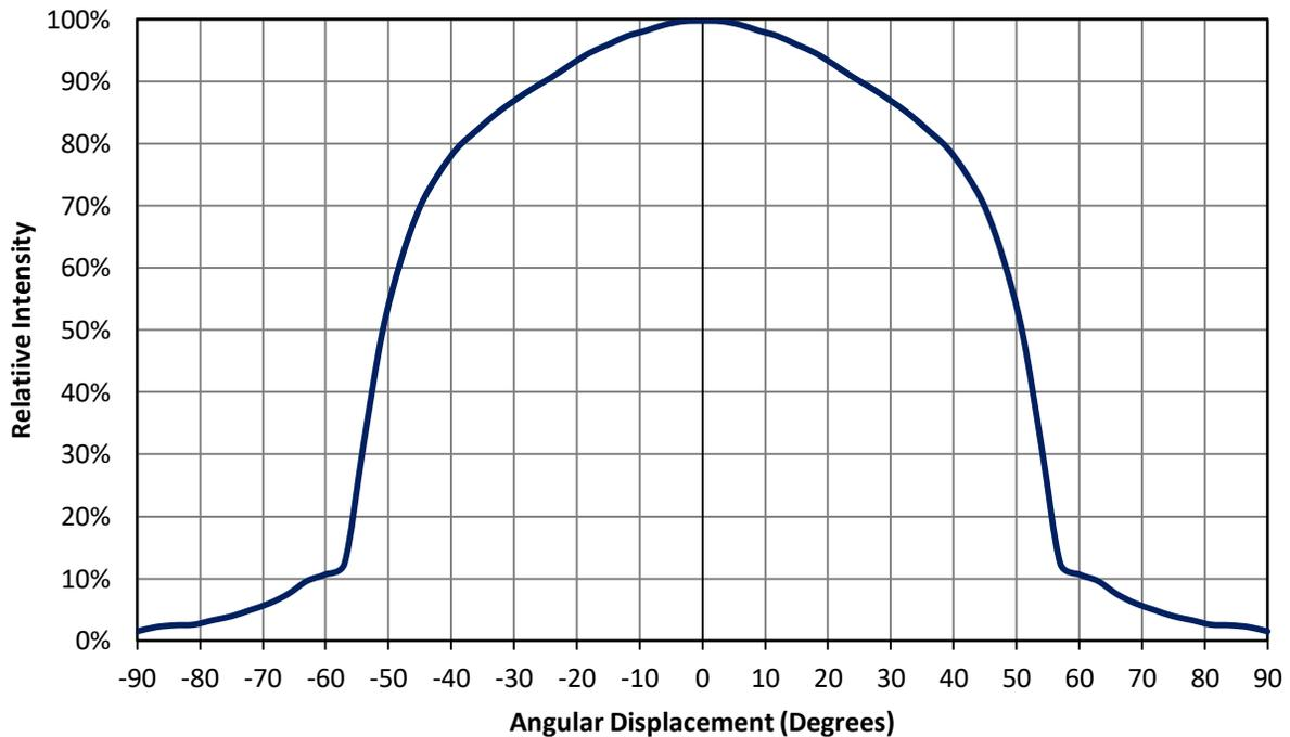
Figure 4: Typical representative spatial radiation pattern @ T<sub>c</sub> = 25°C.
