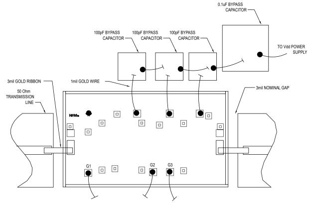
Note: Vgg1, Vgg2 and Vgg3 must be connected to RF/DC ground.
