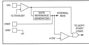
When power is applied to the circuit and VIN is below the upper UVLO threshold,  $I_{IN}$  will be below  $600\mu$ A, the reference generator will be off, the fault latch is reset, the soft-start pin is discharged, and the outputs are actively held low. When VIN exceeds the upper UVLO threshold, the reference generator turns on. All else remains in the shut-down mode until the output of the reference, VREF, exceeds 4.75V.
