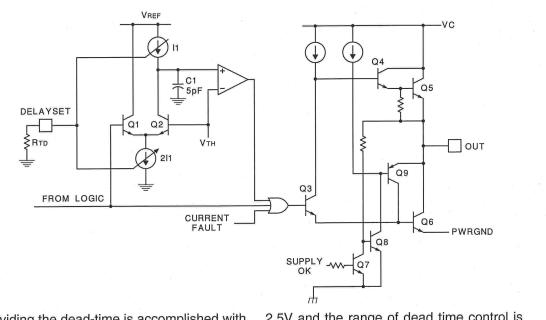
The delay providing the dead-time is accomplished with C1 which must discharge to  $V_{TH}$  before the output can go high. The time is defined by the current sources, I1, which is programmed by an external resistor,  $R_{TD}$ . The voltage on the Delay Set pins is internally regulated to
