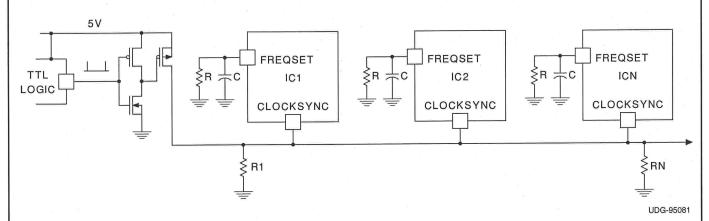
ICs will sync to fastest chip or TTL clock if it is higher frequency.
