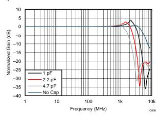
Figure 67. Frequency Response with Capacitive Load
