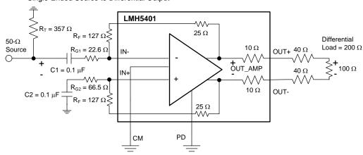
Figure 61. AC-Coupled, Single-Ended Source to a Differential Gain of a 4-V/V
