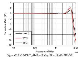
Figure 9. Bandwidth vs Temperature
