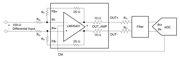
Figure 68. Differential ADC Driver Block Diagram
