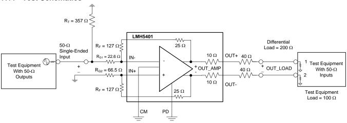
Figure 56. Test Schematic: Single-Ended Input, Differential Output,  $A_V = 4 \text{ V/V}$
