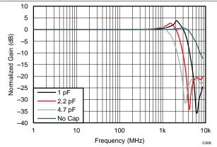
$\rm V_S=\pm 2.5~V,~VOUT\_AMP=2~V_{PP},~capacitance~at~DUT~output~pins,~G=12~dB,~SE-DE$
