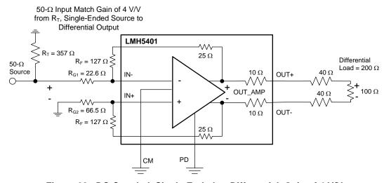
Figure 60. DC-Coupled, Single-Ended-to-Differential, Gain of 4 V/V
