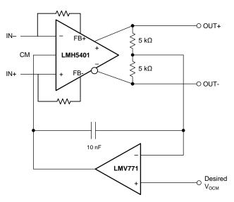
Figure 72. Common-Mode Correction Circuit
