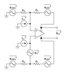
Figure 64. FDA Noise-Analysis Circuit
