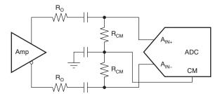
Figure 69. Biasing AC-Coupled ADC Inputs Using the ADC CM Output
