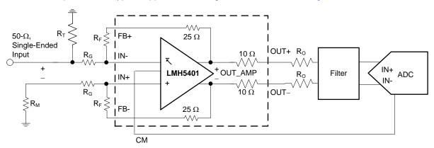
Figure 65. Single-Ended Input ADC Driver
