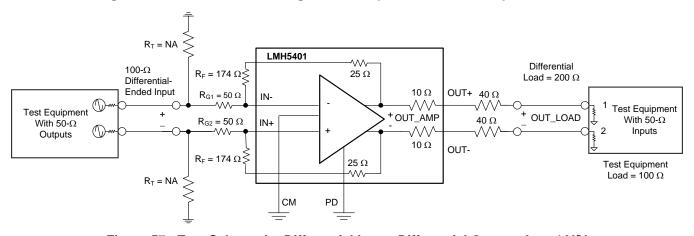
Figure 57. Test Schematic: Differential Input, Differential Output,  $A_V = 4 \text{ V/V}$
