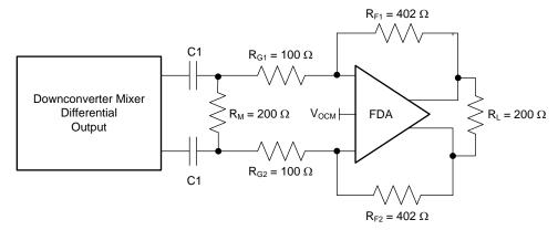
Figure 62. Downconverting Mixer AC-Coupled to the LMH5401 ( $A_V = 4 \text{ V/V}$ )
