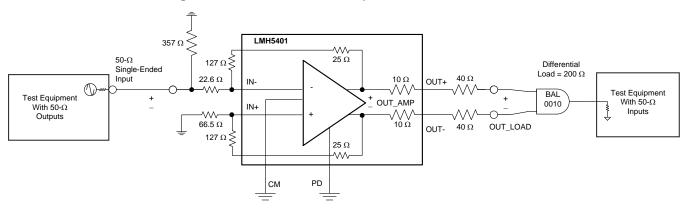
Figure 59. Test Schematic for Noise Figure and Single-Ended Harmonic Distortion,  $A_V = 4 \text{ V/V}$
